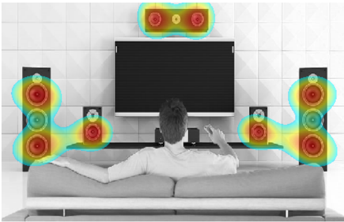
Fig. 8. Simulated image of eight point sources at frequency 3.5 kHz with Nor848A-10 with 50% of elements removed. Image shown with dynamic range 3 dB.
