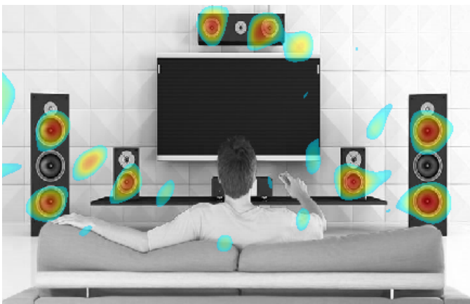
Fig. 4. Simulated image of eight point sources at frequency 3.5 kHz with sparse ring array with 50% of elements removed. Image shown with dynamic range 3 dB.
